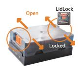
Our sample rack uses a *LidLock* lever to secure the top of the rack. The *LidLock* can prevent the tubes in racks from falling out if the rack is inverted or dropped. Simply push the *LidLock* in the desired direction as marked by the arrows to open or lock the rack.
